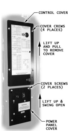
Figure 4.7. Loosen Cover Screws
