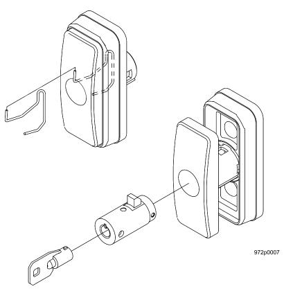
6. Leave the door open and test the lock mechanism with a key. Do not close the door until you are certain the key will unlock the lock.
