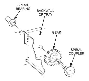
b. Install the spiral coupler. (See "Install a Gear" on page 28).
