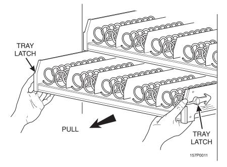
2. Push the tray toward the back of the cabinet. The tray latches on the sides of the tray will lock into position.
