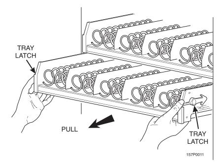
4. Continue pulling the tray forward for another inch. You will then be able to tilt the tray downward into the loading position as shown. The candy or snack tray is now ready for loading.
