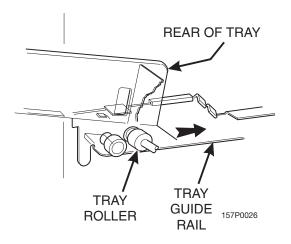
5. Lift up on the tray and slide it toward the back. No more than an inch should be needed
