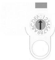
To start, the LED should be lit green and the rotary switch in position 0.
