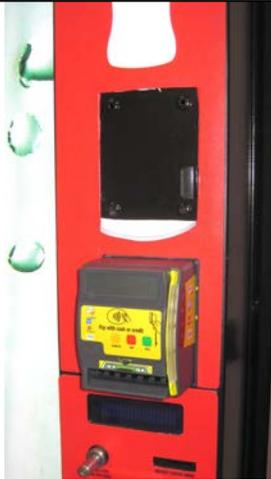
Note: On this particular install, the hole in the mounting plate is partially blocked by the vending machine wall.
