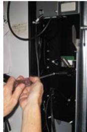
Use the screws removed from the Blocker Plate to install the IVDS Touch Screen Large mounting plate.
