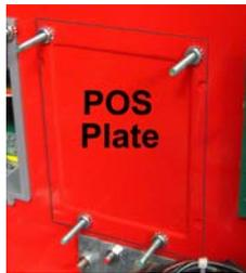
Remove the POS knockout plate
